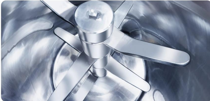
Figure 2: Example of the tool configuration in the heating mixer. Source: Mixaco
