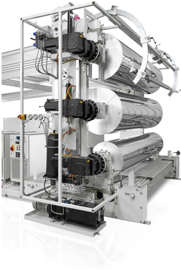
Figure 4: Calender for Sheet Production
